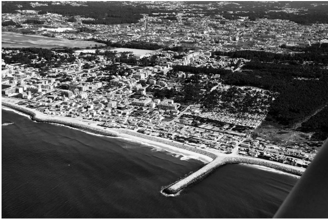
Figure 3. NW coast of Portugal. The urban fronts of Esmoriz and Cortegaça, in the southern part of Porto, are stabilised artificially, are deprived of sediment, and thus do not permit bathing (courtesy of Lopes, 2010).
